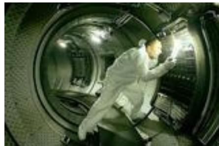
A technician checks a plasma heating system inside a chamber of the Tore Supra nuclear reactor in Cadarache, France, the site proposed by the EU for the International Thermonuclear Experimental Reactor, a prototype of a nuclear fusion reactor based on the Tore reactor. The 25 EU member countries have brought Japan under pressure by confirming that they are ready to build the reactor without Japanese cooperation in case of a disagreement over the final project's site location.
